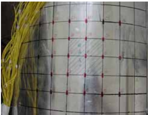
图 8 铝套筒模型及内表面应变片位置 Fig.8 Aluminum sleeve-like model and strain-gage distribution
