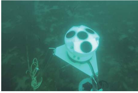
图2 ADCP现场布置情况 Fig. 2 ADCP site placement and layout
